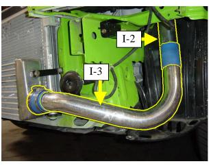
(4) Install the I-4 to the intercooler outlet as shown. (Parts Used #: 5, 13)
