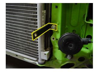
(2) Mount the Intercooler as shown using provided hardware. Secure the left side of the intercooler (looking from the front of the vehicle) to the bracket installed in the previous step.
