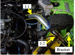
(3) Install the I-3 pipe between I-2 and intercooler inlet as shown.
