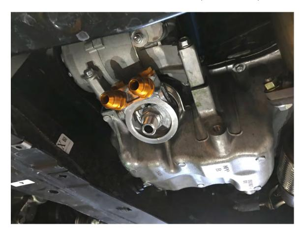
2.2 Install new oil filter to the GReddy Sandwich Adapter Block as shown.
