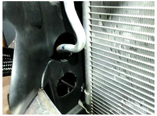
2.6 Install the Bracket #1 and #2 to the GPP x Koyo Oil Cooler core and mount it to the Factory bumper reinforcement beam as shown. (Parts used #1,6,7,8,9)
