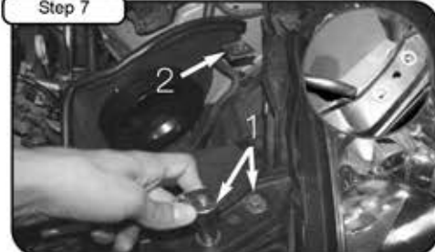
1) Loosen the 2, 12mm bolts on radiator support, place new housing into vehicle. (guide housing tabs into slot between radiator support and OE ram air) Re-Tighten the two bolts. 2) Place bolt from step 3, and tighten using 10mm socket.
