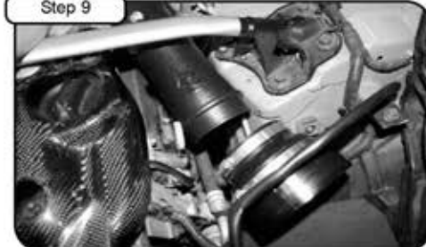
Place coupler reducer on filter adapter with clamps provided, and install tube under OE strut tower bar, keep loose to allow repositioning.
