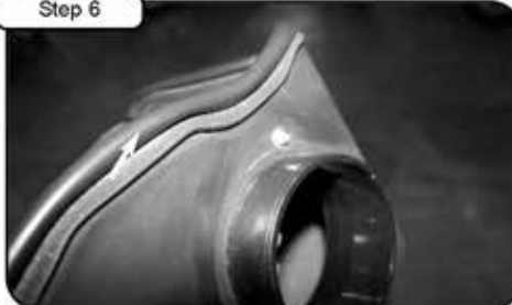
Install 7/16" trim seal to housing. Install filter adapter to housing using button head screws and washers provided.
