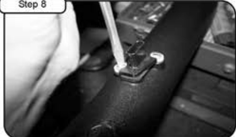
Remove MAF sensor from OE airbox using phillips screwdriver. Re-install to new aFe tube with hardware provided (make sure gasket and nylon spacers are between tube and sensor) using flat head screwdriver.
