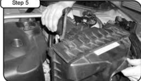
Carefully lift, and remove OE airbox out of vehicle.
