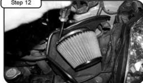
Place high FLOW filter into housing and tighten using 5/16" nut driver.
