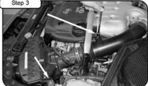
Remove stock intake with 10mm socket. With 10mm socket remove the 2 bolts holding in OE airbox. Disconnect the MAF sensor harness. Save 1 bolt.
