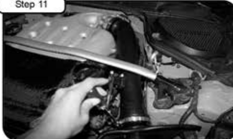
Install straight coupler to throttle body with clamps provided, and tighten all clamps with 5/16" nut driver. Re-connect MAF sensor harness.
