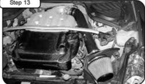
Your installation is now complete. Check all clamps and hoses periodically. Thank you for choosing GReddy!
