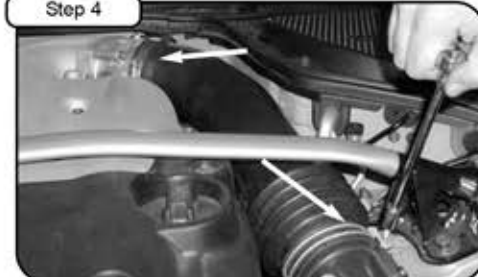
With 10mm socket, loosen the two clamps holding in OE intake. Remove crank case breather from intake tube. Remove Intake tube.
